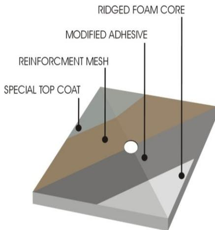
Our pre-sloped Shower Base Boards are made the same way as the Construction Board. With the same characteristics: strong, waterproof, and water resistant, easy to install. And work with.
