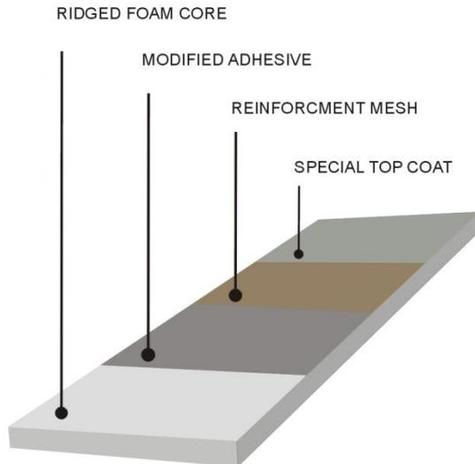
The foam core ensures outstanding thermal insulation properties and high compressive strength with very low weight.
